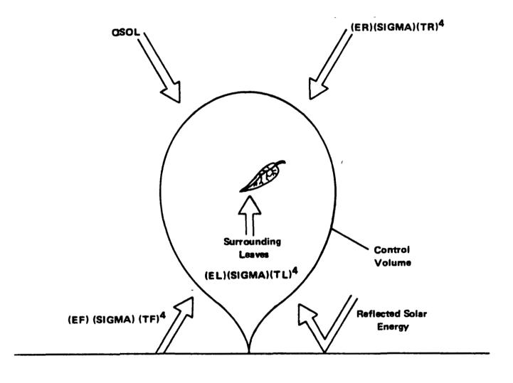
FIGURE 2. RADIATIVE HEAT TRANSFER TERMS INCLUDED IN THE LEAF ENERGY BALANCE
