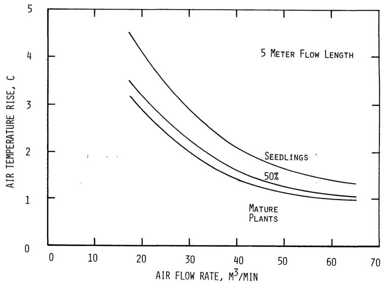
FIGURE 4. AIR TEMPERATURE RISE THROUGH PLANT GROWTH MODULE
