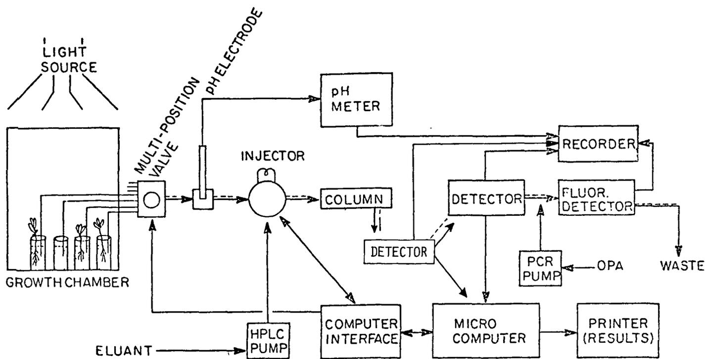
Figure 1. Flow diagram for determining uptake kinetics of N species by wheat seedlings. Detector 1 is a UV absorbance detector set at 189 nm for determination of urea. Detector 2 is a UV detector set at 210 nm for determination of  $\text{NO}_3^-$  and  $\text{NO}_2^-$ . Detector 3 is a fluorescence detector used for  $\text{NH}_4^+$  determination.
