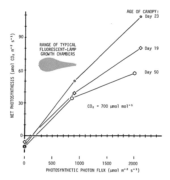
Figure 1 Net photosynthesis as a function of irradiance level. Note that photosynthesis of a dense canopy increases with increasing light at least up to the level of sunlight. Note also that most growth chambers in use today (which use fluorescent plus incandescent lamps; PPF about 250 to 900  $\mu$ mol m-2 s-1) are just above the light compensation point. At such a light level, doubling the irradiance more than doubles net photosynthesis.
