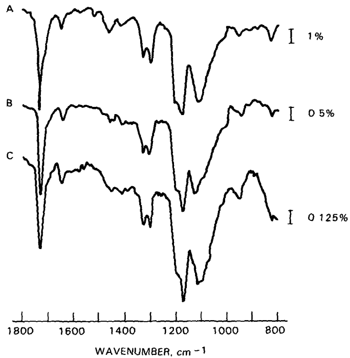
Figure 16. Infrared Spectra of Y-MPS Films with Three Different Thicknesses Deposited on Aluminum Mirrors
