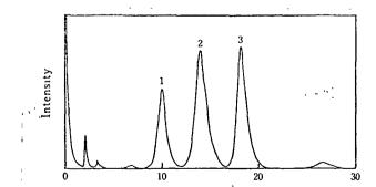
Retention time (min) Fig. 1 Gas chromatogram of esterified products (Meesters) Column : Silicone DC 550 (20%)/Celite 545 (60~80 mesh)
