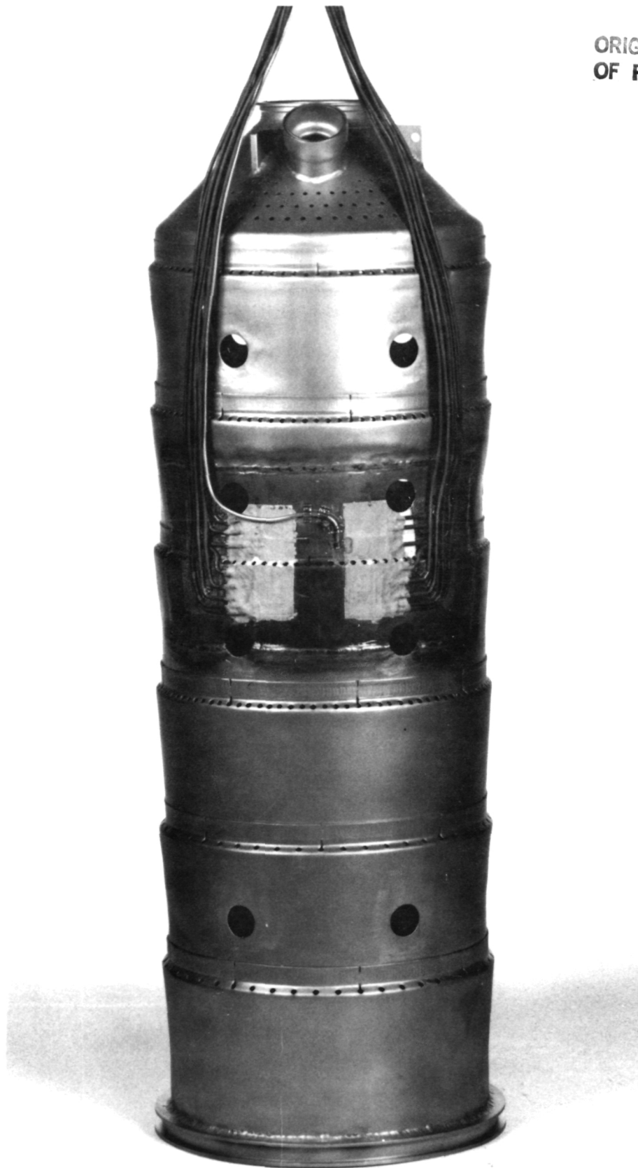
FIG. 11 BURNER CAN WITH INSTRUMENTED SECTION REINSTALLED
