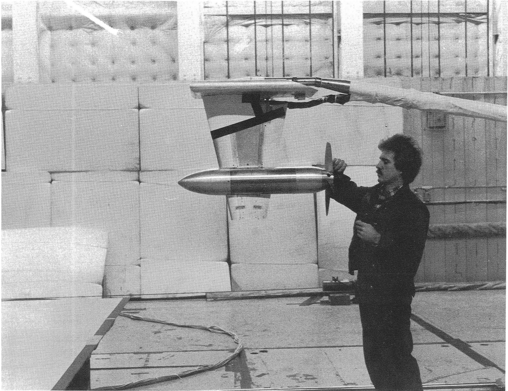
Figure 3.- Photograph of pylon-mounted pusher propeller/nacelle.
