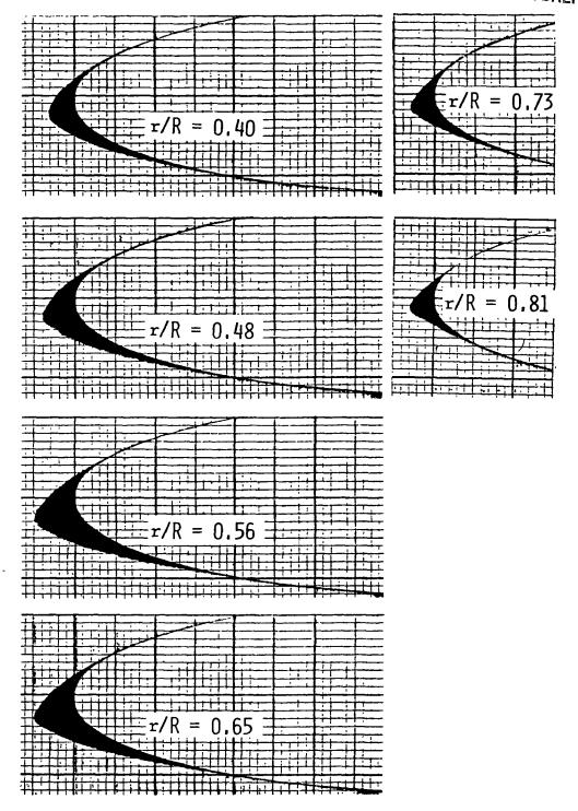
FIGURE 4. PROJECTIONS OF MOLDS OF ICE ACCRETIONS IN LEVEL FLIGHT ( FLIGHT H )
