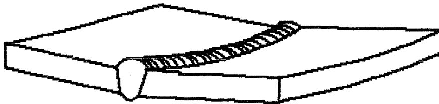
Figure 5. Shrinkage distortion in a butt weld. This distortion includes peaking and longitudinal curvature.
