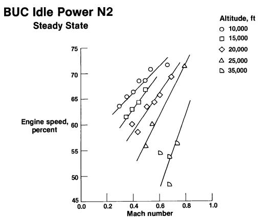
Idle-to-military power BUC transients were performed at various altitudes. The figure below shows the transients that were performed. These transients were snaps and throttle ramps of 3, 5, and 7 sec. The purpose of performing the transients was twofold — to determine the limits where and when compressor stalls occur, and to determine the BUC throttle rate limits for future control designs.
