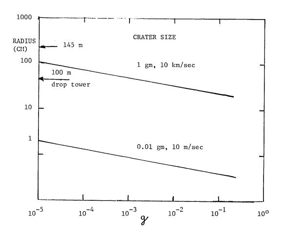
Figure 1. Calculated Ottawa sand crater diameter at different g levels for a 1 gm iron projectile impacting at  $10\,\mathrm{km/sec}$  and a 0.01 gm plastic projectile impacting at 10 m/sec. Available drop tower dimensions are indicated.
