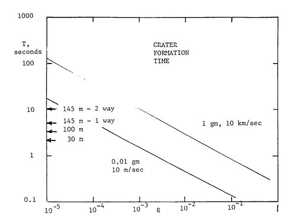
Figure 2. Calculated Ottawa sand crater formation times at different g levels for the two projectiles of Fig. 1. Drop tower test times are indicated.
