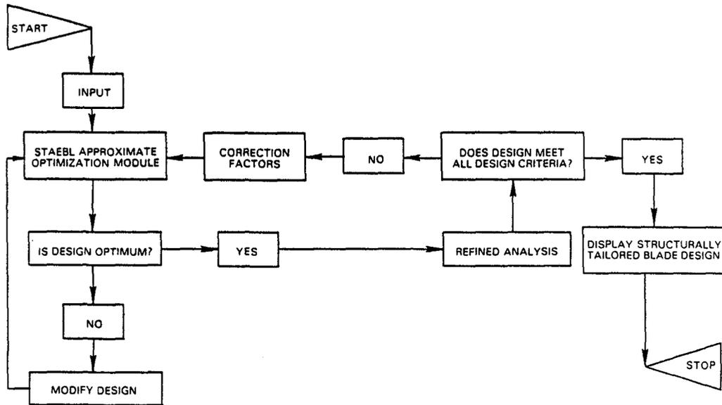
Figure 1 Flowchart for the STAEBL Optimization Process
