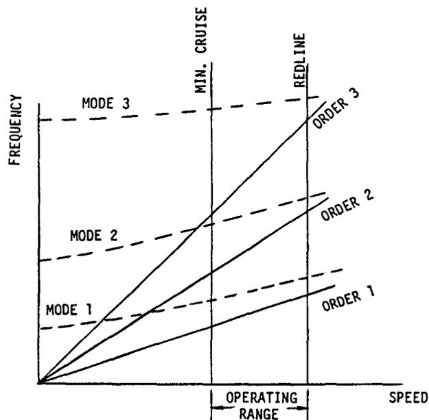
Figure 10 Resonance Diagram for a Successfully Tuned Blade (No Response Crossings Within 5 Percent of the Speed Operating Range)
