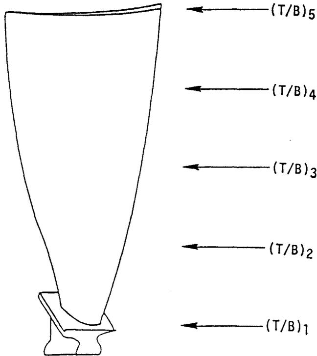
Figure 9 Typical Station Locations for Airfoil Maximum Thickness Starting Values
