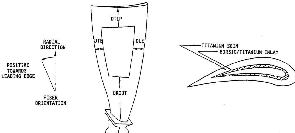
Figure 13 Dimensions and Layup Associated With a Hollow Blade Design
