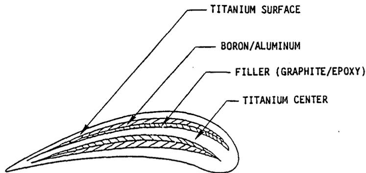
Figure 14 Layup Associated With a Superhybrid Blade Design
