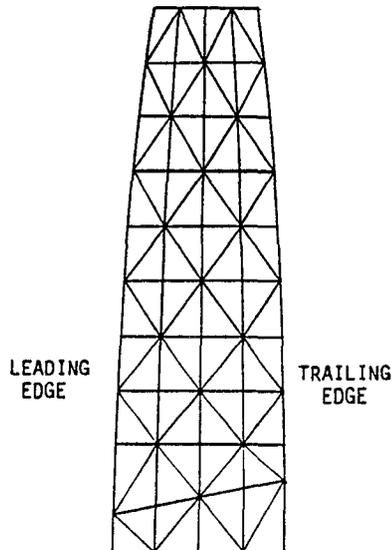
Figure 6 Blade Model With Attachment and Flowpath Angle After Blade Preprocessing
