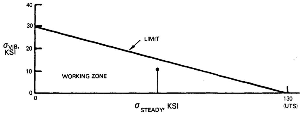
Figure 7 Location of the Worst Vibratory and Steady Stress Combination on the Modified Goodman Diagram - STAEBL
