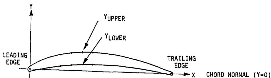
Figure 4 1X2Y Airfoil Section Coordinate Input
