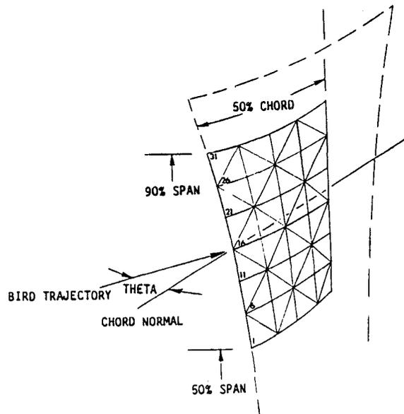
Figure 11 Local Foreign Object Damage Model
