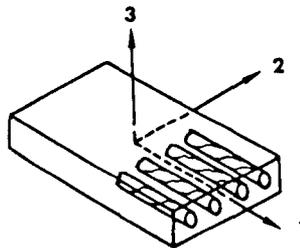
Figure 12 Unidirectionally Reinforced Lamina
