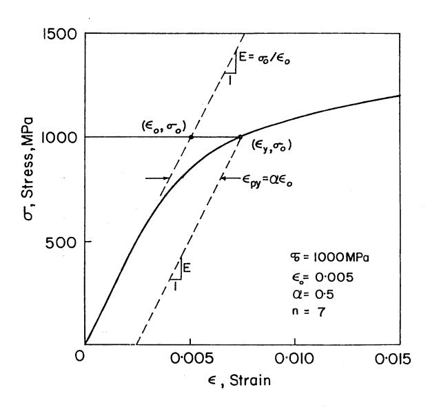
Fig. 2 - Illustration of a uniaxial stress-strain curve.
