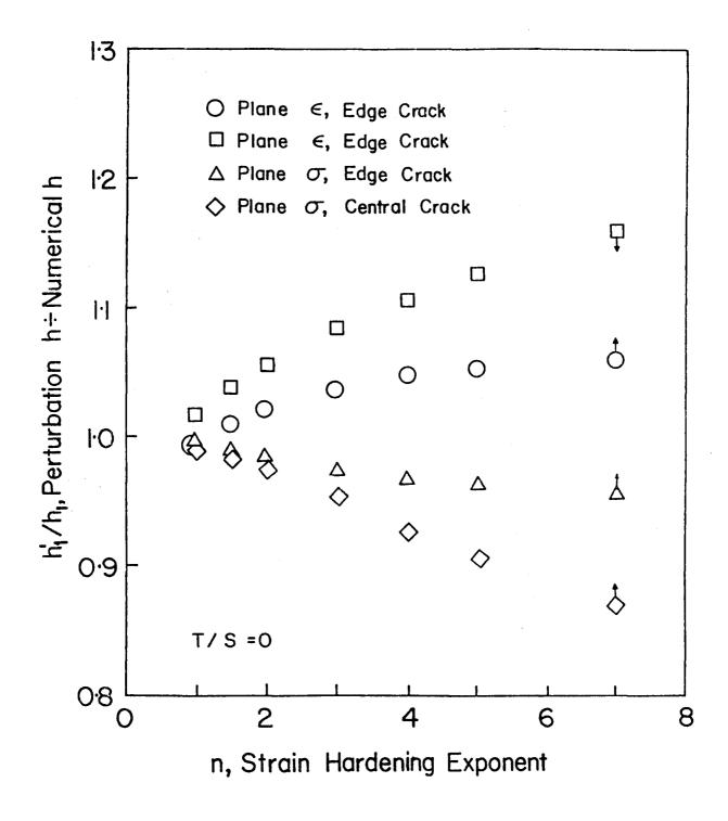
Fig. 4 - Comparison of J-integral constants from He and Hutchinson for edge cracks under plane strain, and for central and edge cracks under plane stress. The numerical  $h_1$  values are either upper or lower bounds - see arrows.
