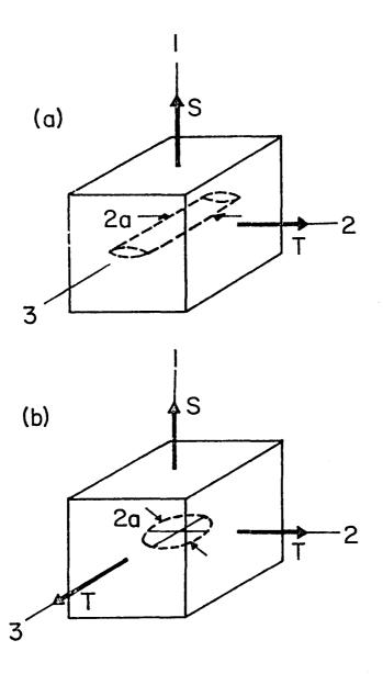
Fig. 1 - Cracked body configurations considered: (a) Two dimensional cases, either plane stress ( $\sigma_3$  = 0) or plane strain ( $\varepsilon_3$  = 0). (b) Circular crack under axisymmetric loading. Bisecting (a) along the 1-3 plane describes cases of two dimensional edge cracks, and bisecting (b) along the 1-3 plane gives a half-circular surface crack.
