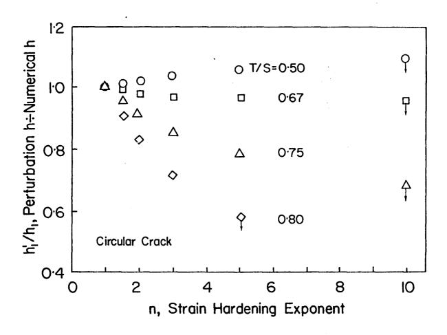
Fig. 6 - Comparison of J-integral constants from He and Hutchinson for circular cracks under axisymmetric loading with in-plane tension. The numerical  $\mathbf{h}_1$  values are all lower bounds - see arrows.
