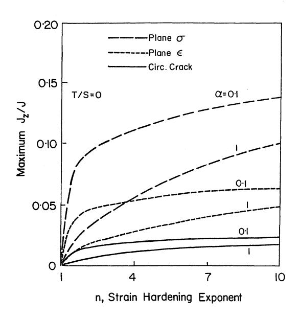
Fig. 12 - Effect of geometric constraint on the plastic zone correction term for uniaxial loading of central cracks in plane stress and plane strain and of circular cracks.
