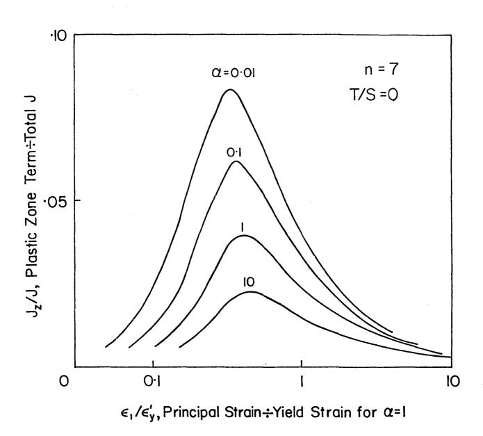
Fig. 11 - Effect of choice of  $\alpha$  on the plastic zone correction term for an interior crack under plane strain.
