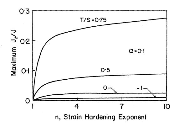
Fig. 13 - Effect of multiaxial loading on the plastic zone correction term for circular cracks under axisymmetric loading.
