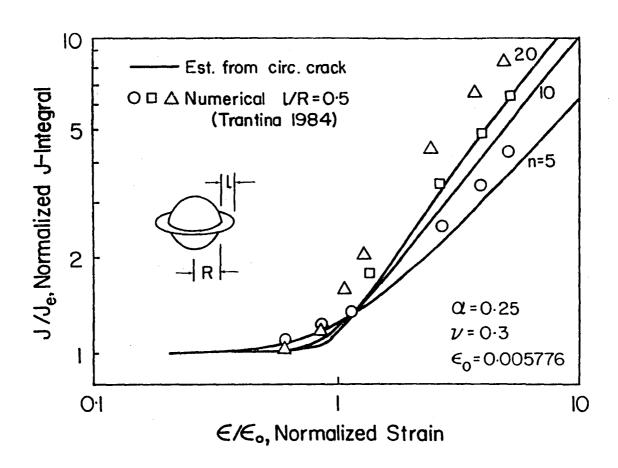
Fig. 10 - Numerical results for a circumferential crack at a spherical void under uniaxial loading compared to estimates based on a circular crack.
