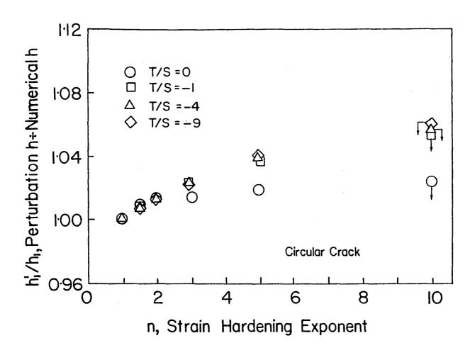
Fig. 5 - Comparison of J-integral constants from He and Hutchinson for circular cracks under axisymmetric loading, either uniaxial or with in-plane compression. The numerical  $h_1$  values are all lower bounds - see arrows.
