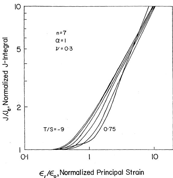
Fig. 7 - J-integral versus strain for various axisymmetric loadings applied to a circular crack.
