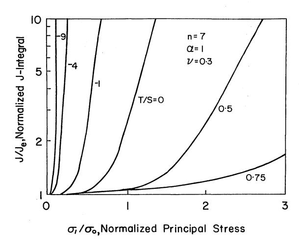
Fig. 8 - J-integral versus stress for various axisymmetric loadings applied to a circular crack.
