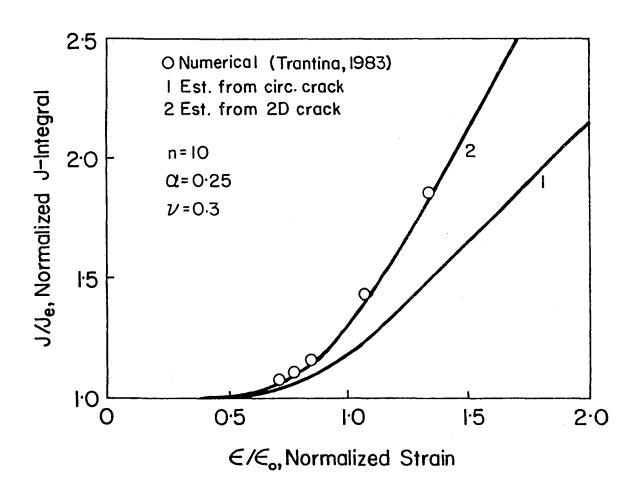
Fig. 9 - Numerical results for a half-circular surface crack under uniaxial loading compared to two estimates.
