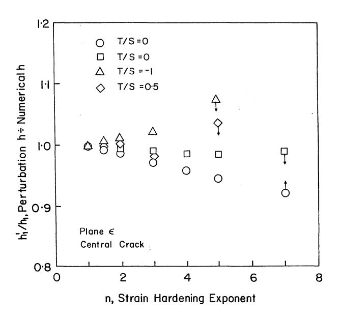
Fig. 3 - Comparison of J-integral constants from He and Hutchinson for central cracks under plane strain. The numerical  $\mathbf{h}_1$  values are either upper or lower bounds - see arrows.
