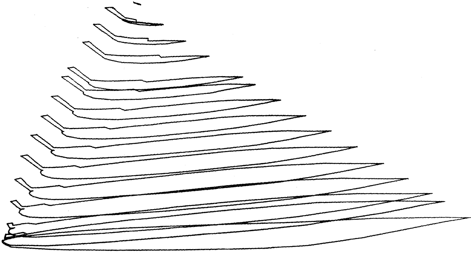
Fig. 8. Streamwise cuts through the wing-flap combination.
