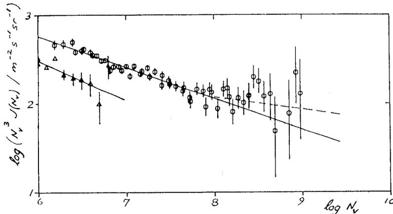
Figure 2. Differential equivalent vertical muon number ( $N_v$ ) spectrum obtained by combining the various muon number spectra at different zenith angles. Line (a) is the maximum likelihood fit to showers with  $\log N_{\mu} < 7.75$  and line (b) is a similar fit for  $\log N_{\mu} > 7.75$ . Each point represents the intensity in a ( $N_{\mu}; \theta$ ) bin. Also shown is the result from the Akeno group ( $1 < \sec\theta < 1.1$ ) and (c) is their fitted line.
