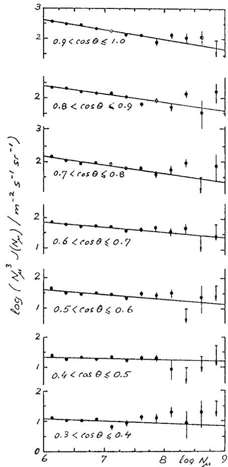
Figure 1. The differential shower size ( $N_\mu$ ) spectra for various zenith angle bins ( $\theta$ ). The ordinate is the flux multiplied by  $N_\mu^3$ . The lines are fitted by maximum likelihood to the lowest seven data points in each range of  $\theta$ .
