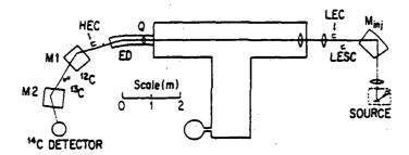
Figure 1. Schematic diagram of system. Abbreviations in the figure are: Minj, injection magnet; LEC, lowenergy Faraday cup (this cup can be moved in and out of the beam); LESC, low-energy side cup; Q, electrostatic quadrupole focus; ED, electrostatic deflector; M1 and M2, high-energy magnets, <sup>13</sup>C and <sup>12</sup>C, high-energy Faraday cups.
