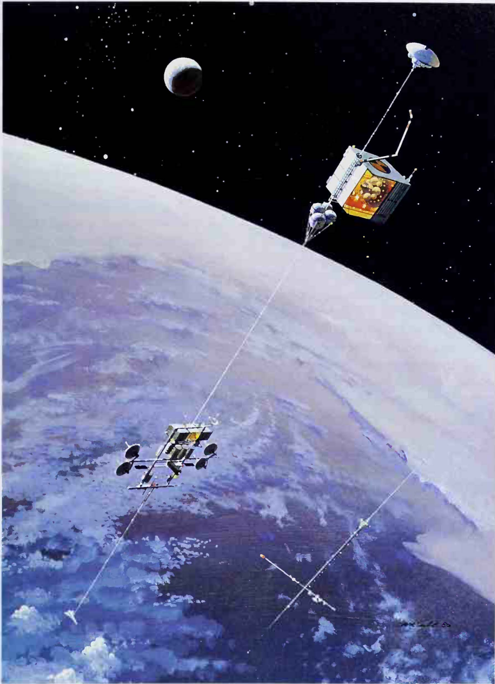
Two space stations in low Earth orbit (LEO) in the early 21st century. In the foreground is an Earth Spaceport with a transfer vehicle being deployed at one end by a tether and a passenger transport vehicle being deployed at the other end in a similar manner. In the background is a Variable Gravity (g) Research Facility that will be used to determine the long-term effects of weightlessness, radiation, etc., on human beings in space. (COURTESY ROBERT MCCALL)
