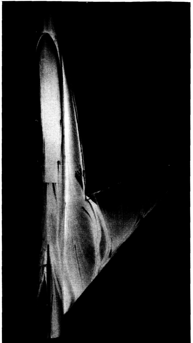
Strake on; \alpha = 7.67^\circ
