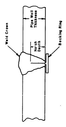
FIGURE 3. NOTCH DEPTH DEFINITION
