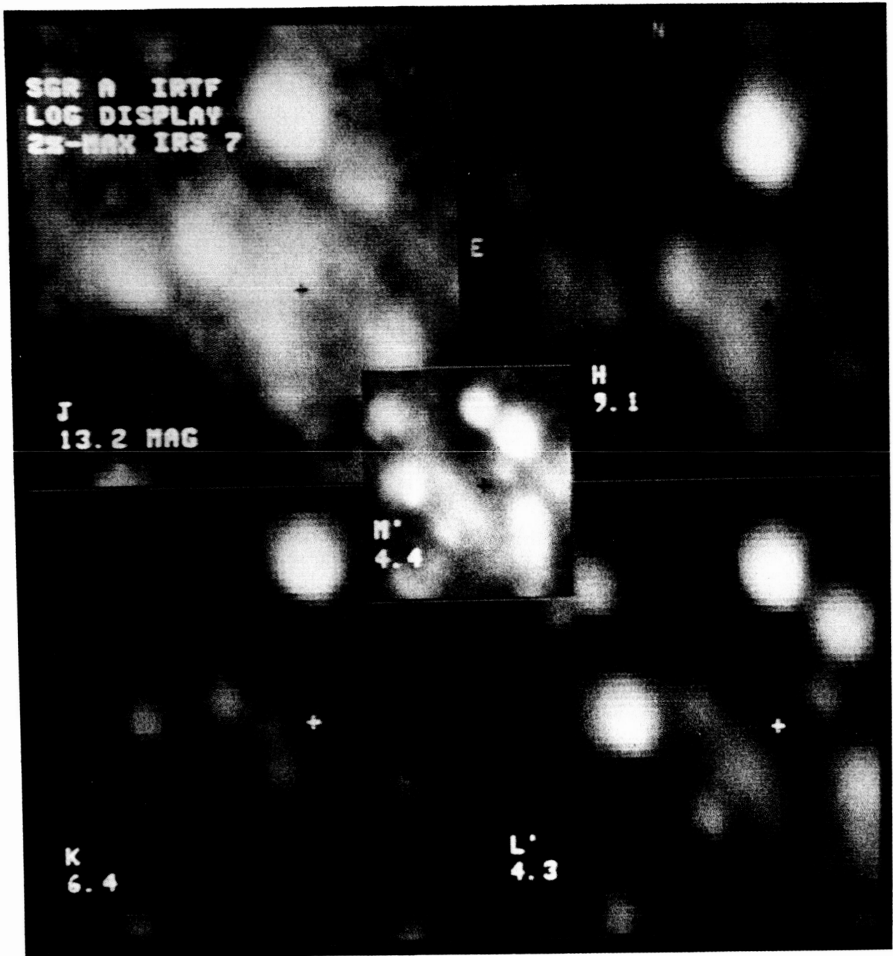
6. 1.23 (J), 2.23 (K), 3.75 (L') and 4.67 (M') micron images of the central regions of the galactic center. The displayed levels are scaled logarithmically from 2% to the peak IRS 7 brightness; the magnitude of IRS 7 is given for reference in each image. A "+" marks the calculated position of Sgr A*. The presence of IRS 3 in the J image may be due to a thermal leak in our J filter.
