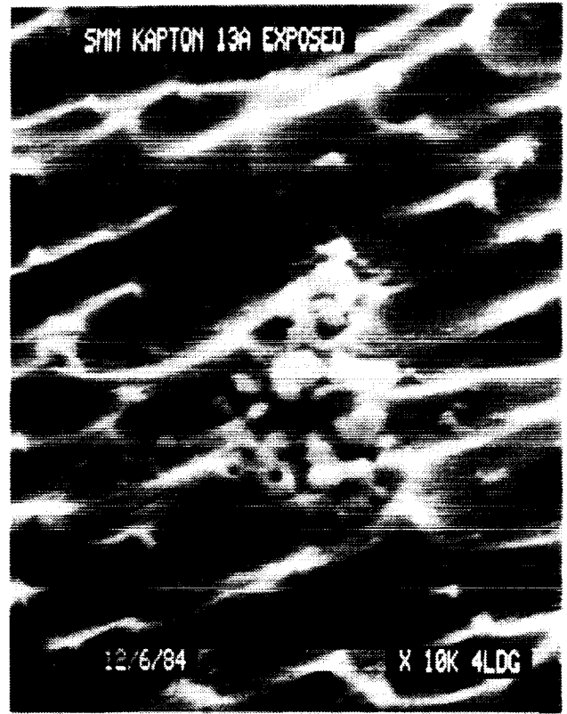
Figure 8 13A Kapton Top layer. The Surface Morphology is Similar to that of the Laboratory Exposed Specimen, but More Erosion Has Taken Place
