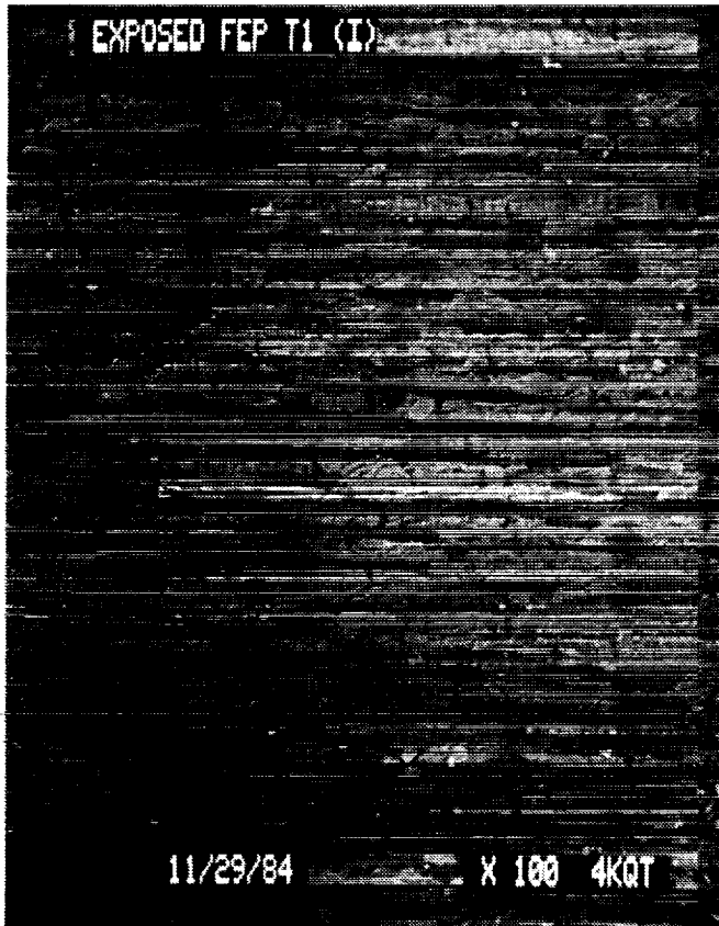
Figure 12 T1 FEP Teflon Exposed Ag/Inconel Side. The Morphology is Similar to that of the Laboratory Exposed Ag/Inconel with Ag Growing Through Cracks and Grain Boundaries in the Inconel Overcoat. At High Magnification it is Possible to Observe Regions in which the Ag/I has been Totally Removed and the FEP Teflon Textured Surface is Visible.
