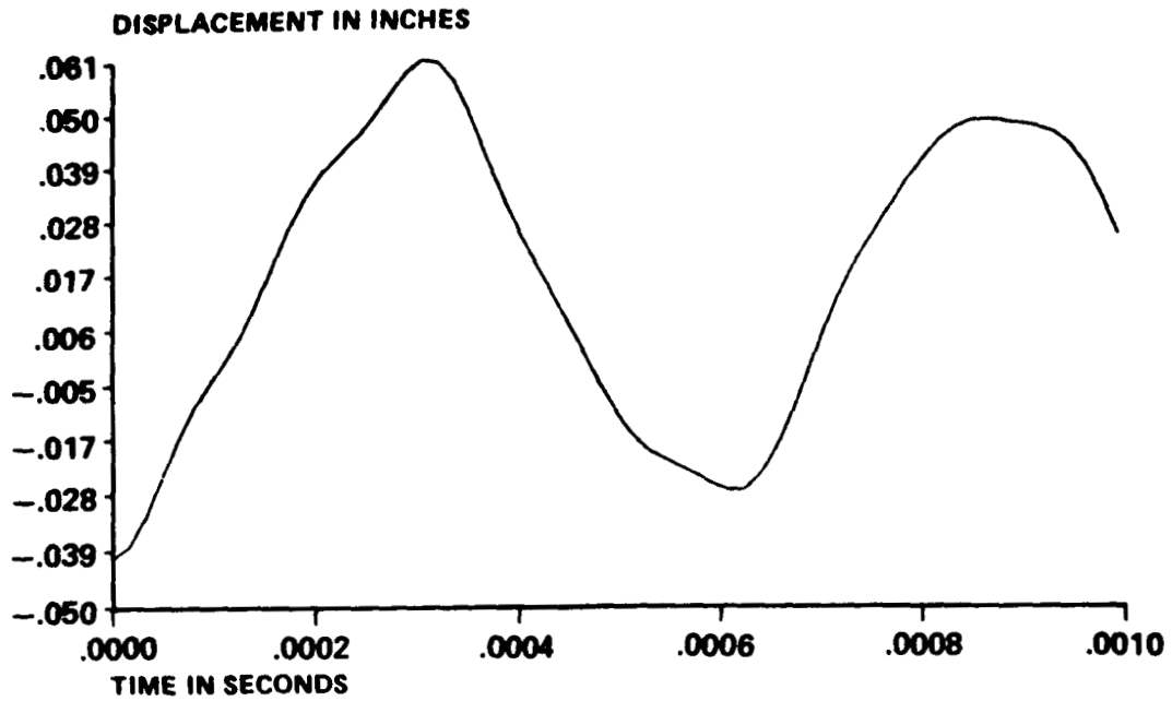
Figure 7. Response of O-ring compressed to 0.046 in. (linear elastic response with pressure).
