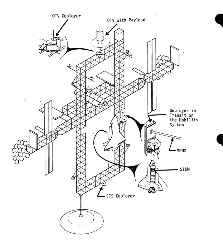
Fig. 1 Space Station with Deployer System
