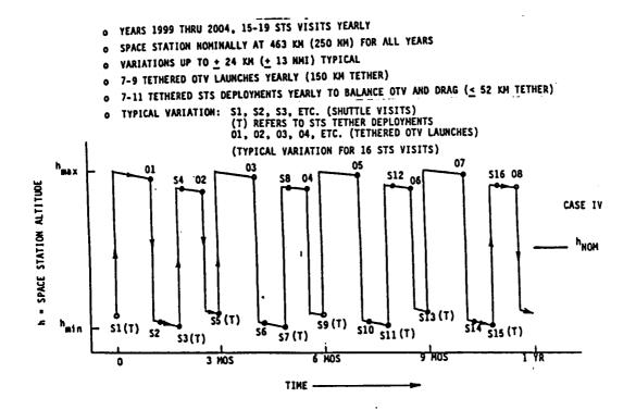
Fig. 4 Momentum Balance - Tethered OTV/STS at Current Altitude
