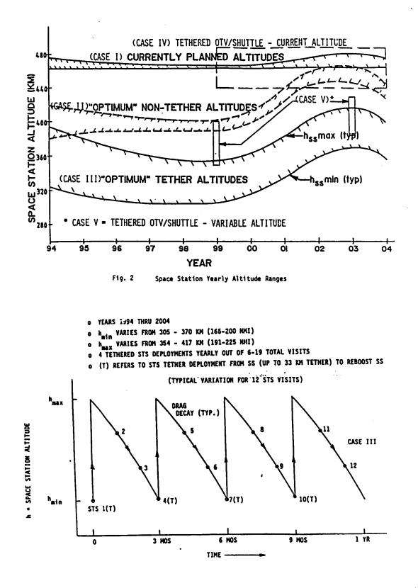
Fig. 3 Homentum Balance - Tethered Shuttle Variable Altitude Operations
