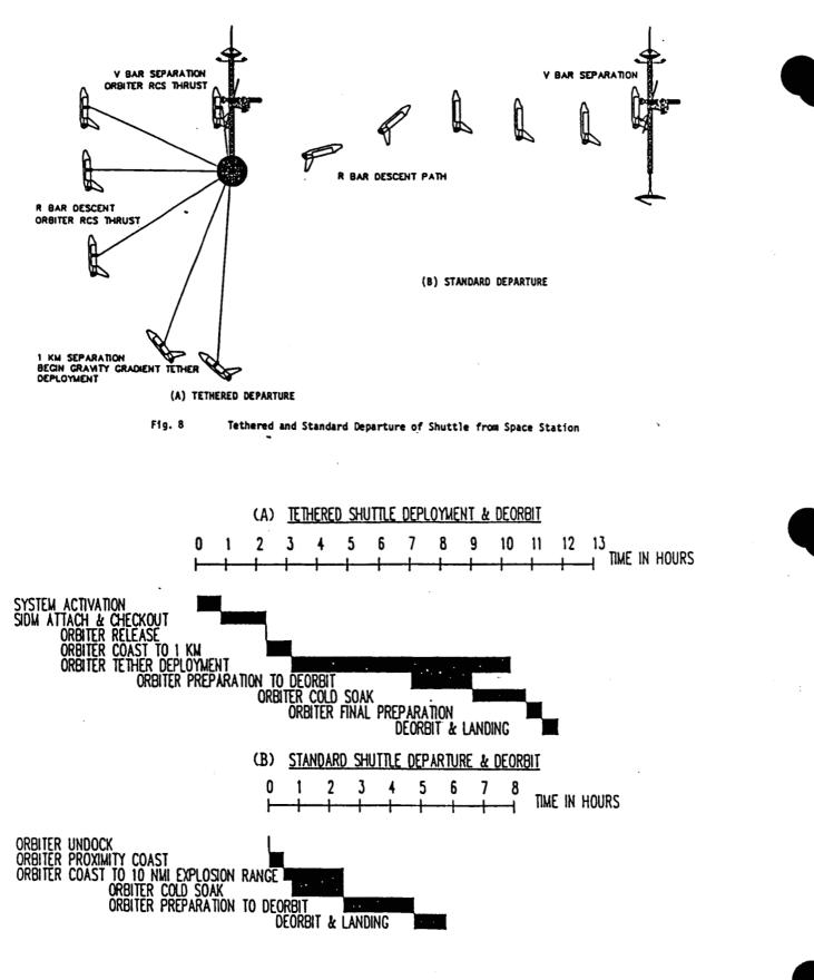
Fig. 9 Tethered and Standard Shuttle Deorbit Timelines
