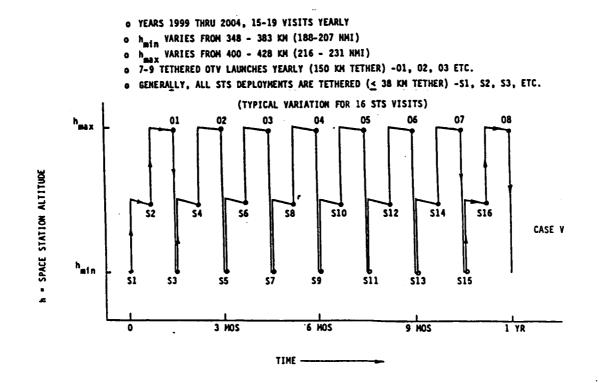
Fig. 5 Nomentum Balance - Tethered OTV/STS at Variable Altitude
