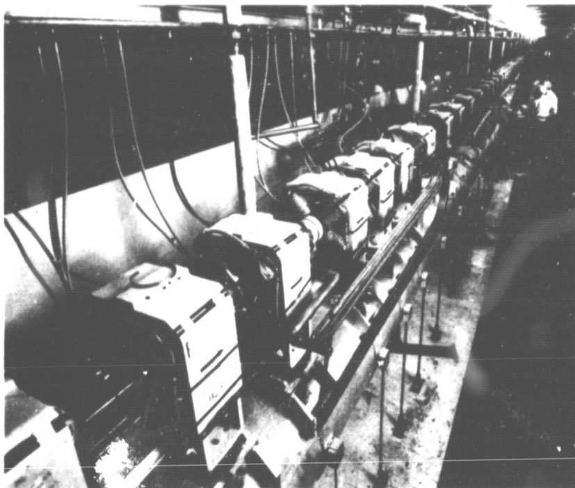
FIGURE 3.5 A view of the 2-mile-long accelerator at the Stanford Linear Accelerator Center (SLAC) looking along the tunnel. The accelerator has just been rebuilt to provide 50-GeV electrons and positrons for the Stanford Linear Collider.
