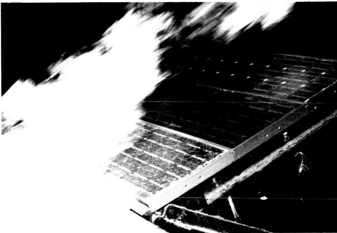
Prototype modules have passed UL 790 Class A burning brand tests which are more severe than this spread of flame test.
