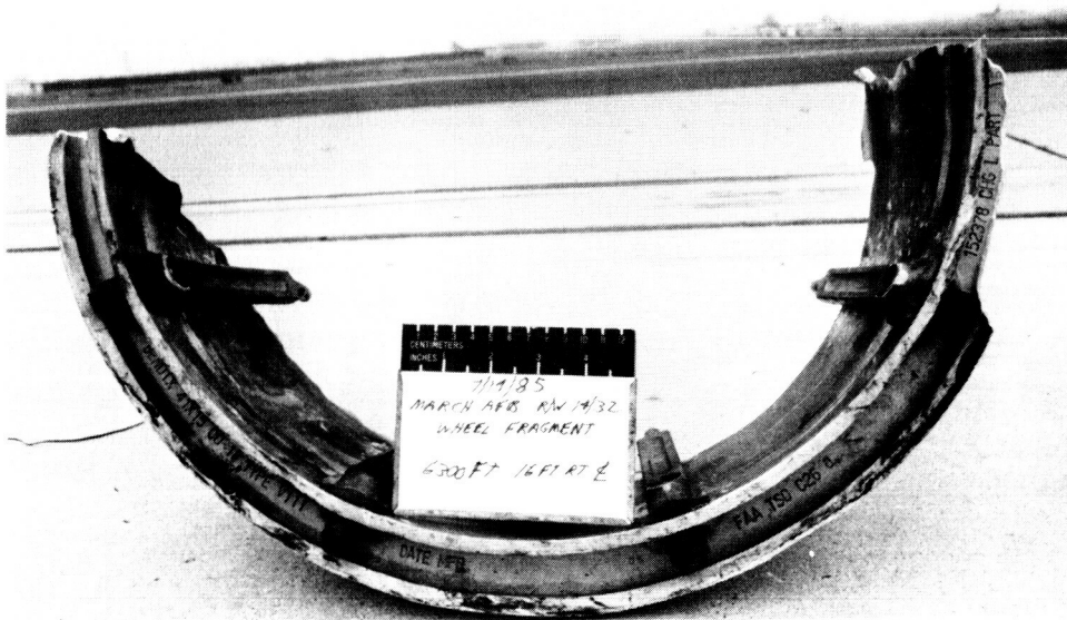
Figure 10. - Fragment of wheel 4 found 6,300 ft from runway 32 threshold.
