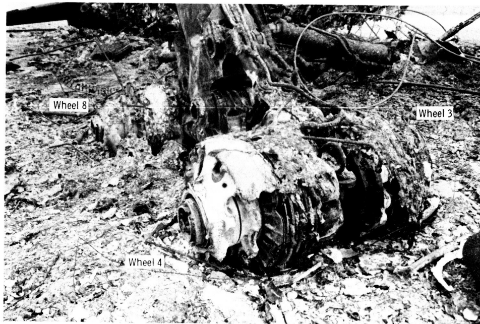
Figure 18. - Closeup view of right main gear wheels after fire.
