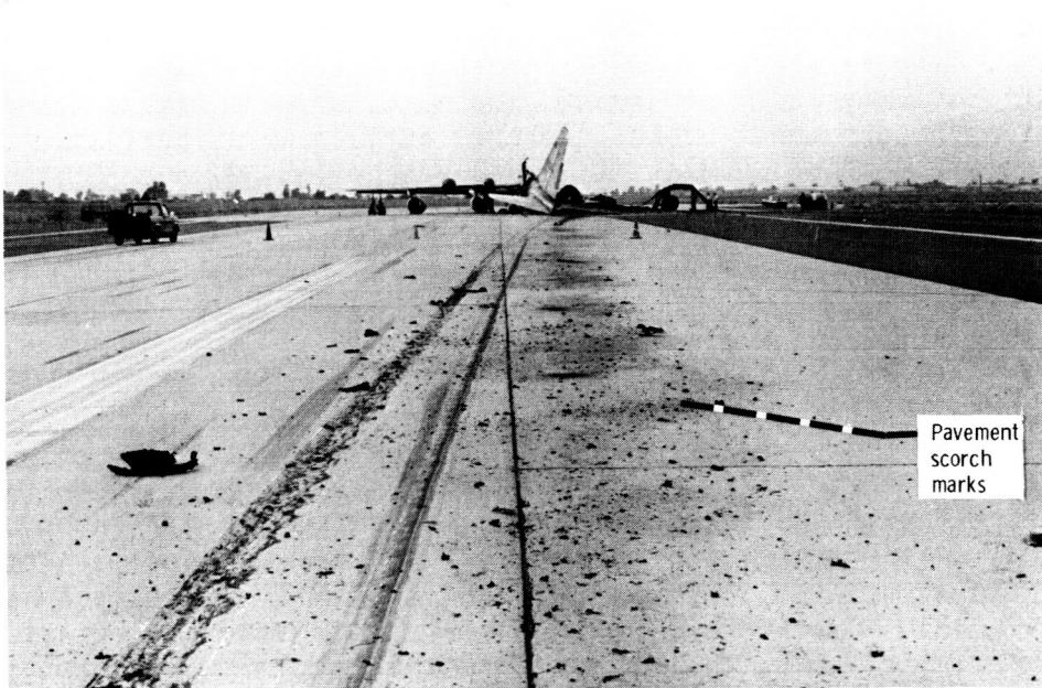
Figure 12. - Runway surface scorch marks and tire rubber debris from right main gear at about 11,950 ft down runway 32.
