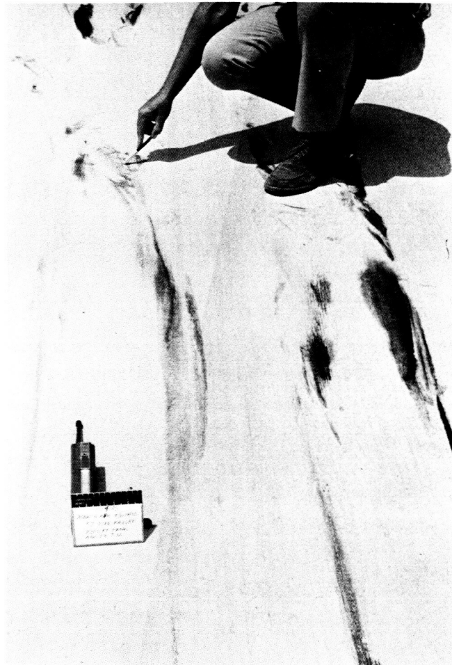
Figure 11. - Runway surface rubber marks from blowout of tire 7.
