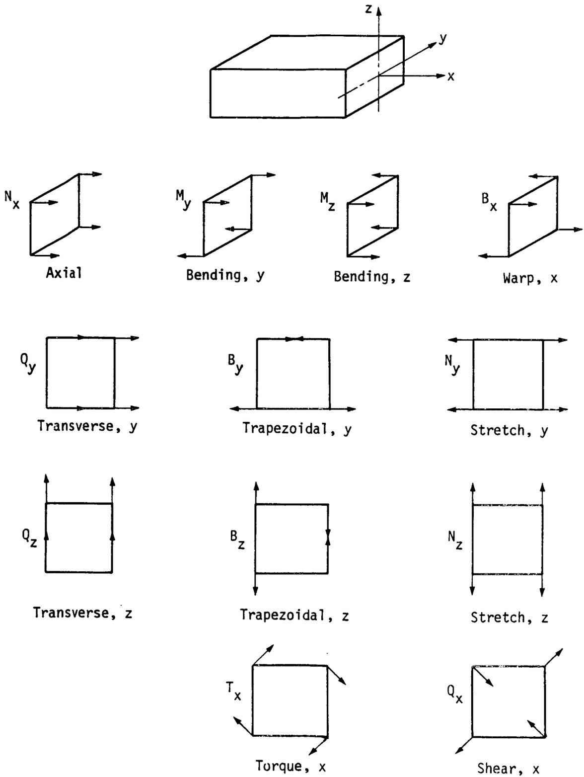
Figure 4 (b). Beamlike Loadings For Square Trusses
