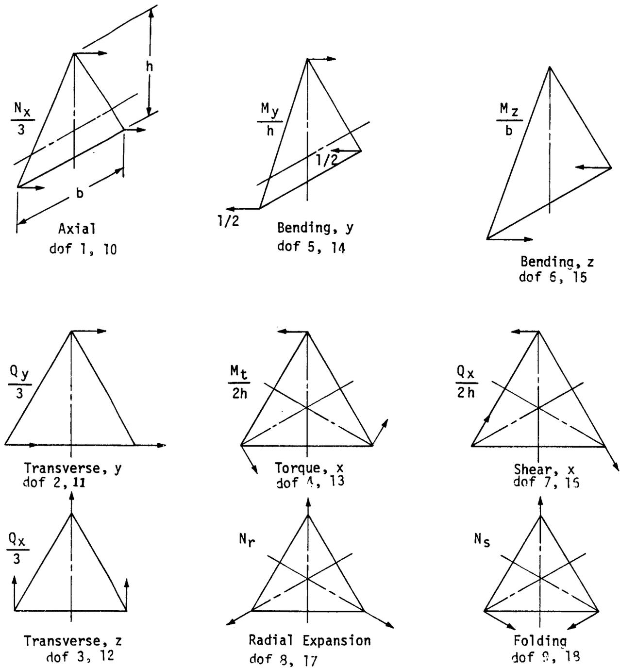
Note: Arrows on Nodes Forces for each Beamlike Loading Condition
