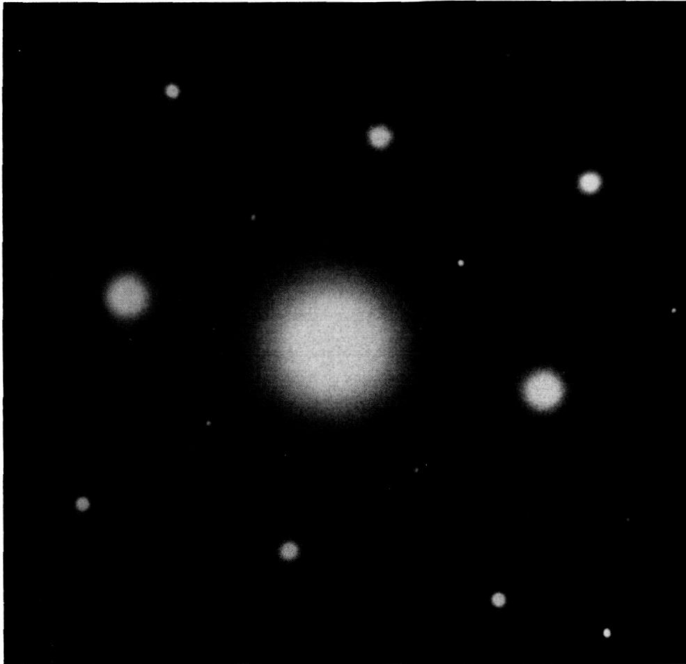
FIGURE 4. - TEM ELECTRON DIFFRACTION PATTERN OF ALGaAs GROWN AT 500 °C WITH THE LASER BEAM (WAVELENGTH 193 NM) IMPINGING.
