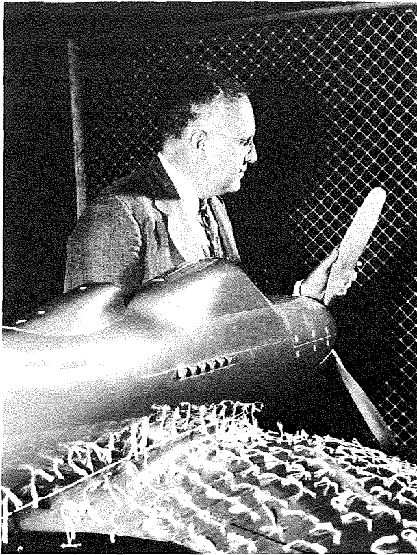
Veteran flight researcher Hartley Soule managed the NACA Muroc Flight Test Unit from his office at Langley. (The model in this photograph was used in tuft survey research. By observing the reaction of the little pieces of cloth, or tufts, attached in various places on the wing, a researcher could tell whether the flow over the surface was smooth or disturbed.)
