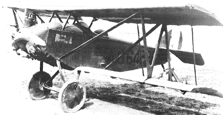
The army's Sperry Messenger airplane with variable-camber wings, 1926.
