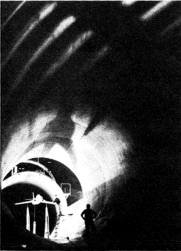
The 16-Foot High-Speed Tunnel at the time of its dedication in 1941. Left, a scale model of a jet airplane being tested in the tunnel during the 1950s.
