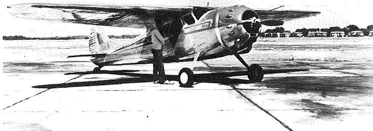
In 1948 this Cessna 190 was used by the NACA to test new ways of controlling the boundary layer at the wing's leading edge.
