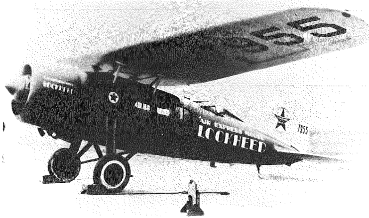
The record-breaking Lockheed Air Express with NACA cowling, 1929.
