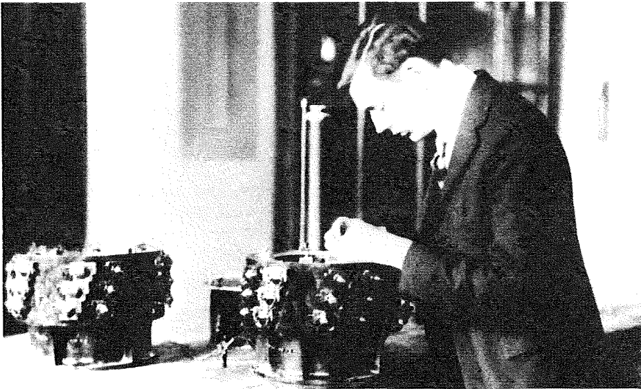
Frederick H. Norton, LMAL chief physicist, observes an airplane flying above his speed course station (top), and works on recording manometers (bottom), about 1922.
