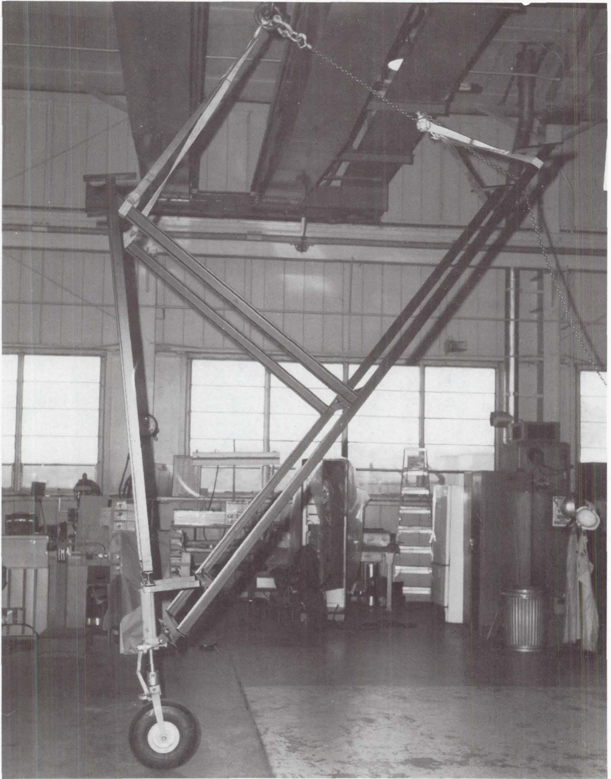
Figure 4. Nose gear and support truss prior to mounting on test carriage.
