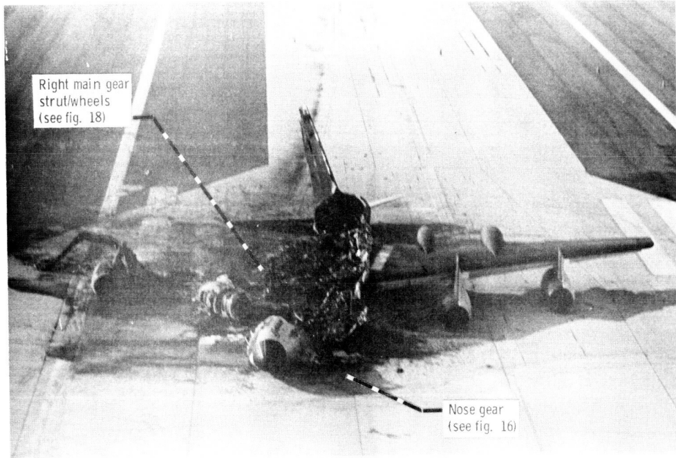
Figure 14. - Aerial view of fire-damaged NASA 712 taken at front of wreckage.
