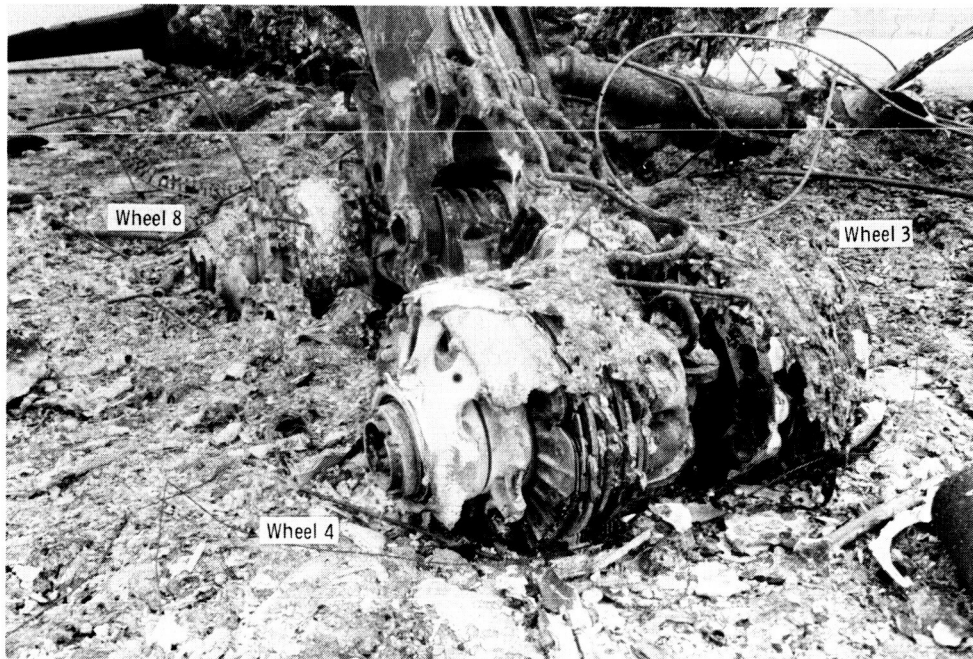
Figure 16. - Closeup view of right main gear wheels after fire.
