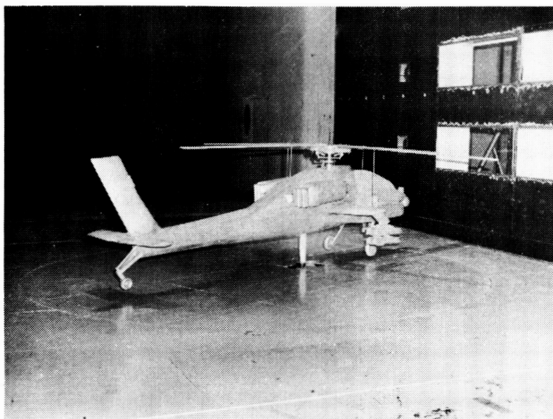
Figure 29. AH-64 "tipover" test installation in the 14- by 22-Foot Subsonic Tunnel.
