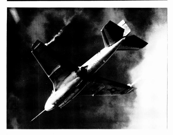
II. In 1979 a modified A-6A aircraft demonstrated the STOL capability of circulation control. This aircraft is shown as it was modified for this proof-of-concept flight demonstration. Externally the modifications included: a tapered cylindrical wing trailing edge, bleed air cross-over duct under fuselage, Krueger flap on the wing gloves, modified leading edge slats and modified horizontal tail.
