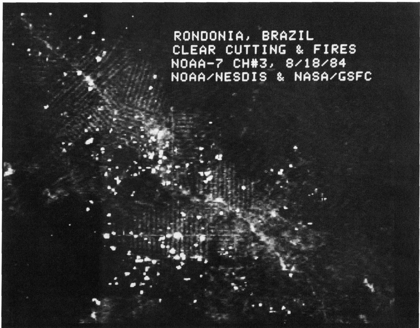
FIGURE 11. This is a NOAA-7 computer-enhanced 3.8 micrometer thermal infrared satellite image of the Rondonia, Brazil area. The image was taken on August 18, 1984 at 19:47 Greenwich Mean Time (GMT) and the resolution is 1.1 kilometers (km). The gray linear features are clear-cut swaths of forest, some more than 80 km long, about 4 km apart, and 600-800 meters wide. The clear-cut area is bisected by highway BR-364. The white areas are fires associated with the clear cutting and slash and burn agricultural activities. The large-scale (100 × 400 km) primary forest disturbance shown in the image is a Government-planned colonization project. Images such as these demonstrate the potential of remote sensing for monitoring deforestation and forest fires.
