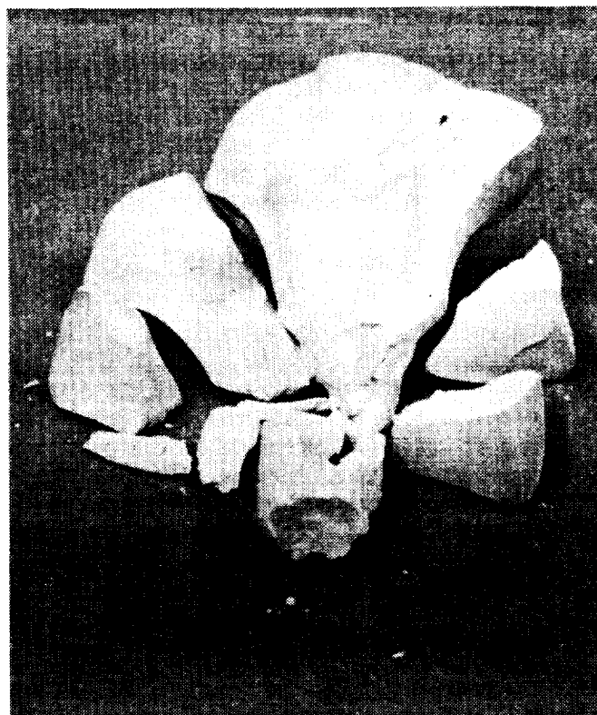
Figure 341. Part After Sintering Cracked Into Several Pieces Due to Incomplete Drying.
