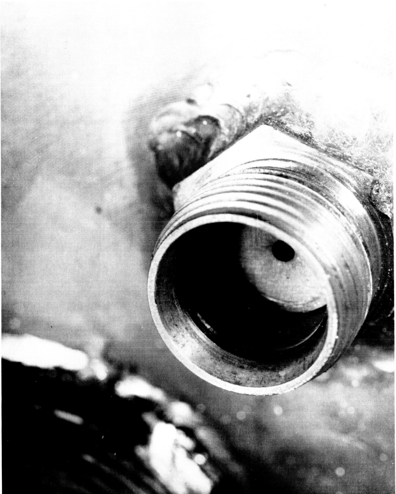
FIGURE 31 UPSTREAM SIDE OF ORIFICE (REF. SAMPLE #3) - POST TEST
