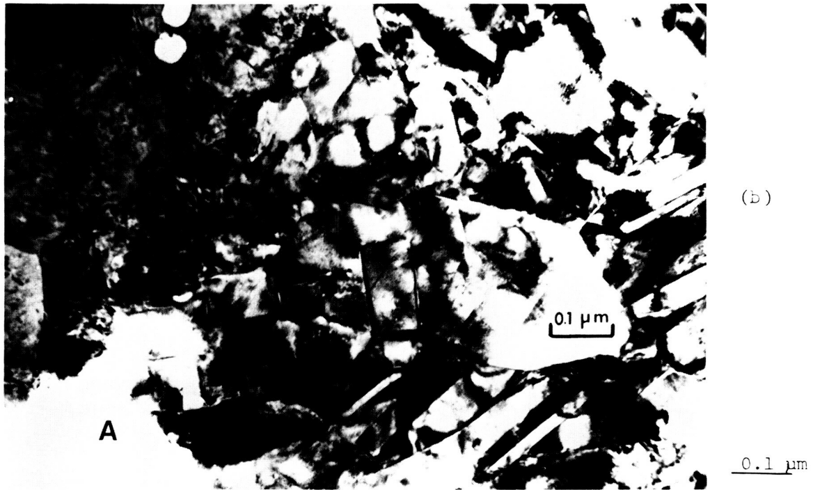
Fig.12. (a)-(b) 19.6% \text{Y}_2\text{O}_3 ceramic coating after 100 hours exposure at 1200^\circ\text{C} (a) monoclinic and cubic grains (b) higher magnification micrograph showing tetragonal grains(A) formed at the interface between monoclinic and cubic grains due to yttrium diffusion.
