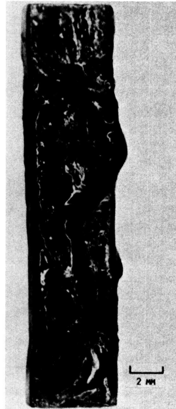
FIGURE 3. - CARBORUNDUM HEXOLOYS SINTERED \alpha - \text{SiC} EXPOSED FOR 40 H AT 1000^\circ\text{C} , 2 PPM Na, 400 KPA (AIR FLOW LEFT TO RIGHT).
