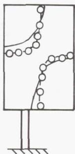
Figure 7. Calculated basic wing mode shapes and measured and calculated node lines.
