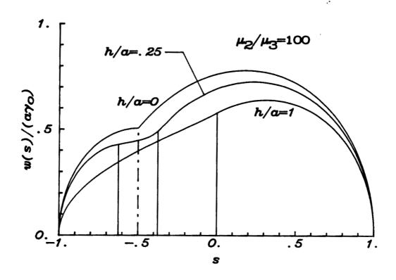
Fig. 3 Normalized crack surface displacement in bonded materials with a nonhomogeneous interfacial zone. In each case shown the crack goes through the zone and the centerline of the zone coincides with the quarter-point of the crack, s=-0.5, where s is the normalized coordinate defined by  $x=s(b_3-a_2)/2 + (b_3+a_2)/2$  (Fig. 1).
