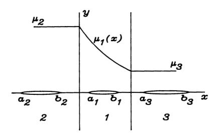
Fig. 1 Geometry of bonded materials containing cracks perpendicular to the nominal interface
