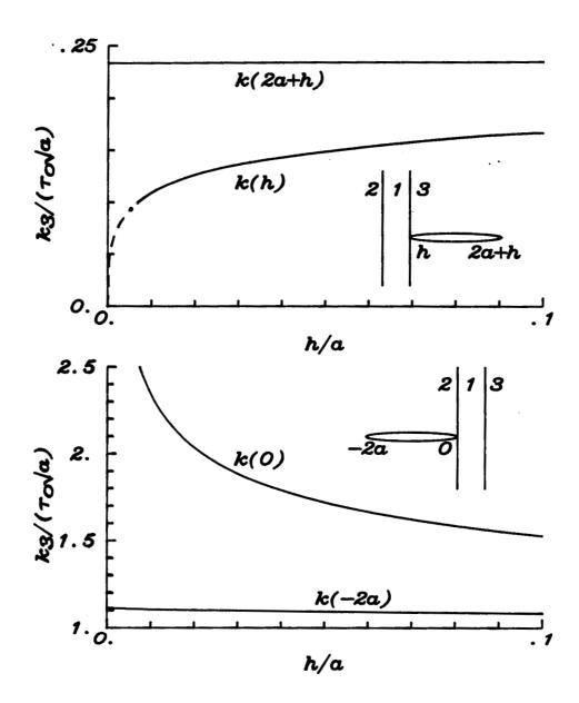
Fig. 2 Normalized stress intensity factors for the crack terminating at the interfacial zone in bonded materials;  $\mu_2=4\mu_3$ ,  $\tau_0=\mu_2\gamma_0$ , where  $\gamma_0$  is the uniform shear  $\gamma_{yz}^\infty$  away from the crack region.
