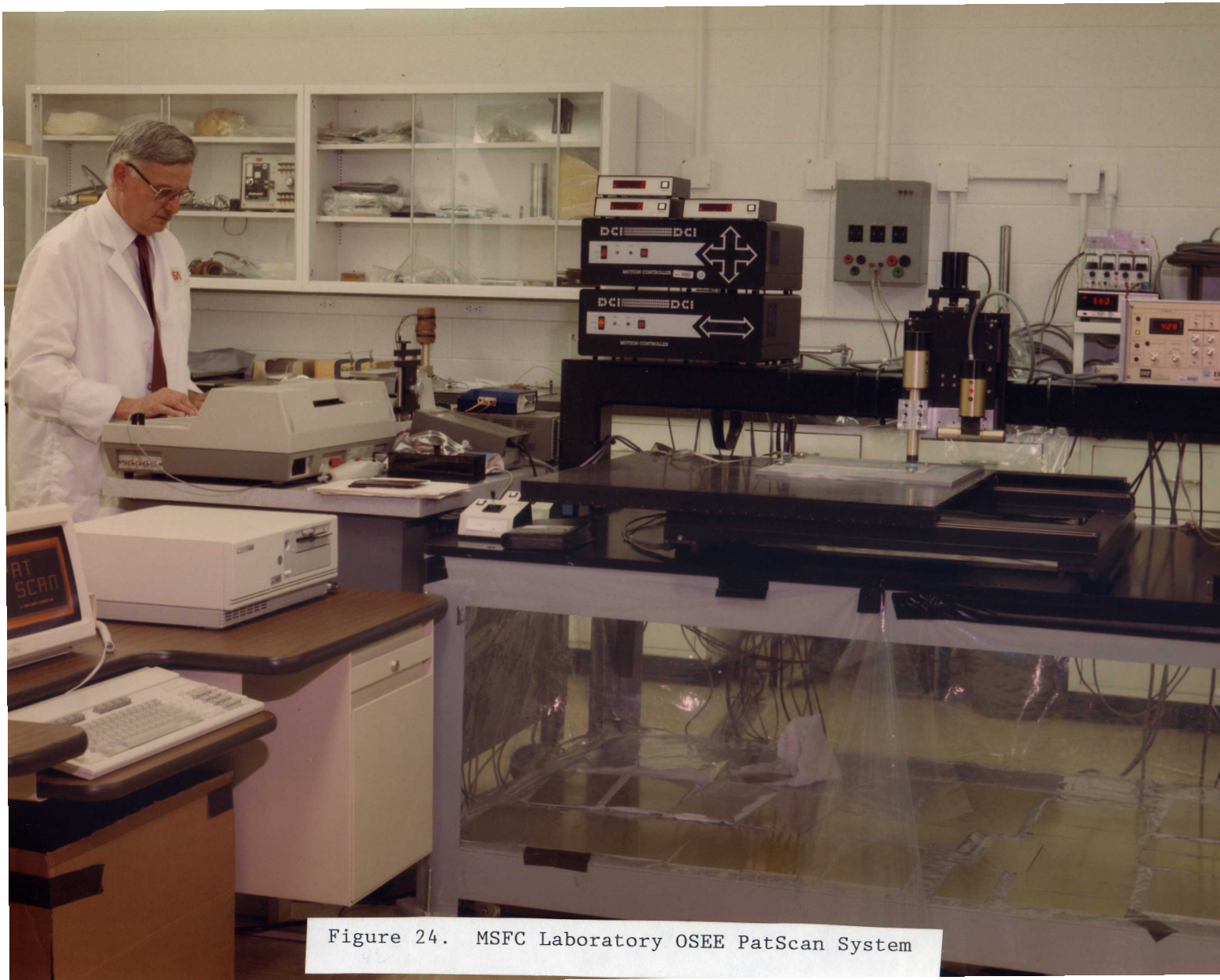
Figure 24. MSFC Laboratory OSEE PatScan system.
