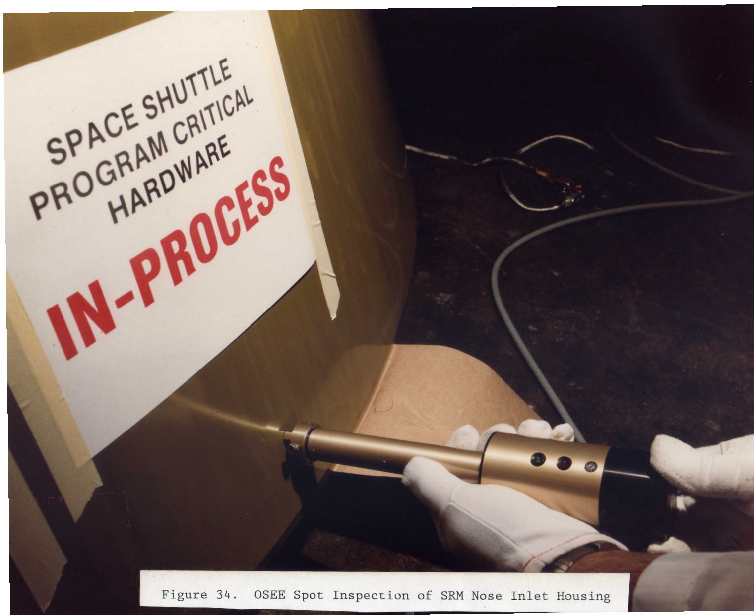
Figure 34. OSEE spot inspection of SRM nose inlet housing.
