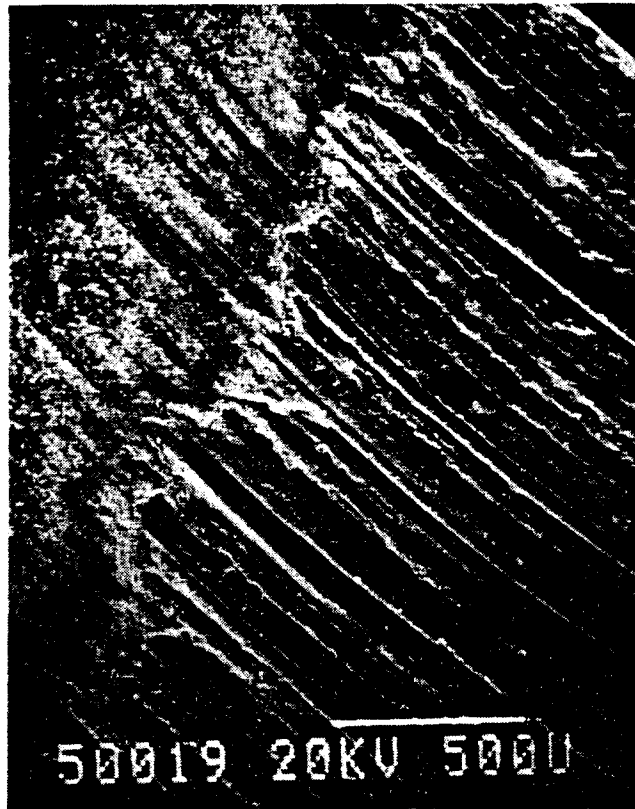
FIGURE 8.15 2024 ALUMINUM, STATOR-SIMULATING RUB SURFACE AFTER 60 SECONDS OF RUB AGAINST THE STEEL SHAFT. MAGNIFICATION: 50 TIMES. PHOTO # 50019.
