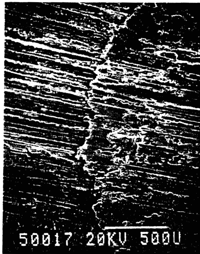
FIGURE 8.13 2024 ALUMINUM, STATOR—SIMULATING RUB SURFACE AFTER 15 SECONDS OF RUB AGAINST THE STEEL SHAFT. MAGNIFICATION 50 TIMES. PHOTO # 50017.
