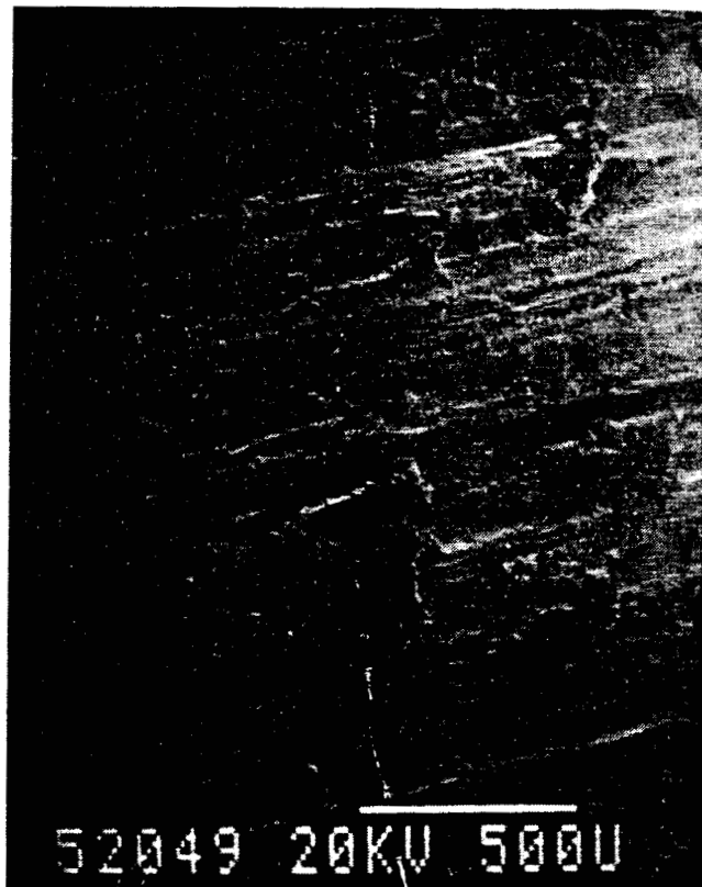
FIGURE 8.22 STEEL ROTOR SHAFT SURFACE AFTER 15 SECONDS OF RUB AGAINST STEEL STATOR. MAGNIFICATION: 50 TIMES. PHOTO # 52049.
