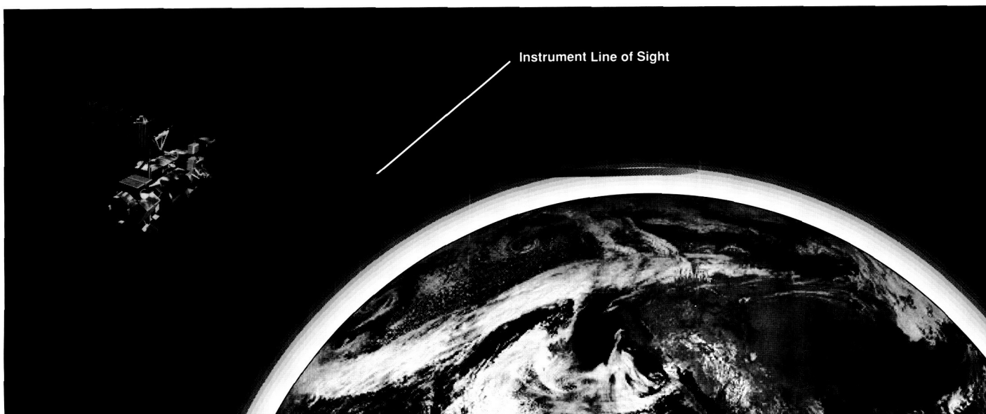
EMISSION MEASUREMENT of trace-gas atmospheric concentration employs limb-viewing geometry to detect characteristic wavelengths of radiation emitted by atmospheric molecules along the line of sight. Intensity of emitted radiation is a measure of the gas density.
