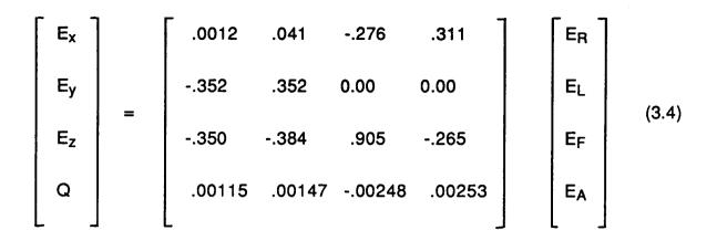
The ideal situation in these two equations would be for each ambient field to be dominated by one of the field mill readings. That is, one would like for one number to be dominant in each row. This would imply that the field mills each respond to only one component of the ambient field or net charge and are recording independent quantities. The above equations clearly do not have this property, which is in any case difficult to achieve in practice.
