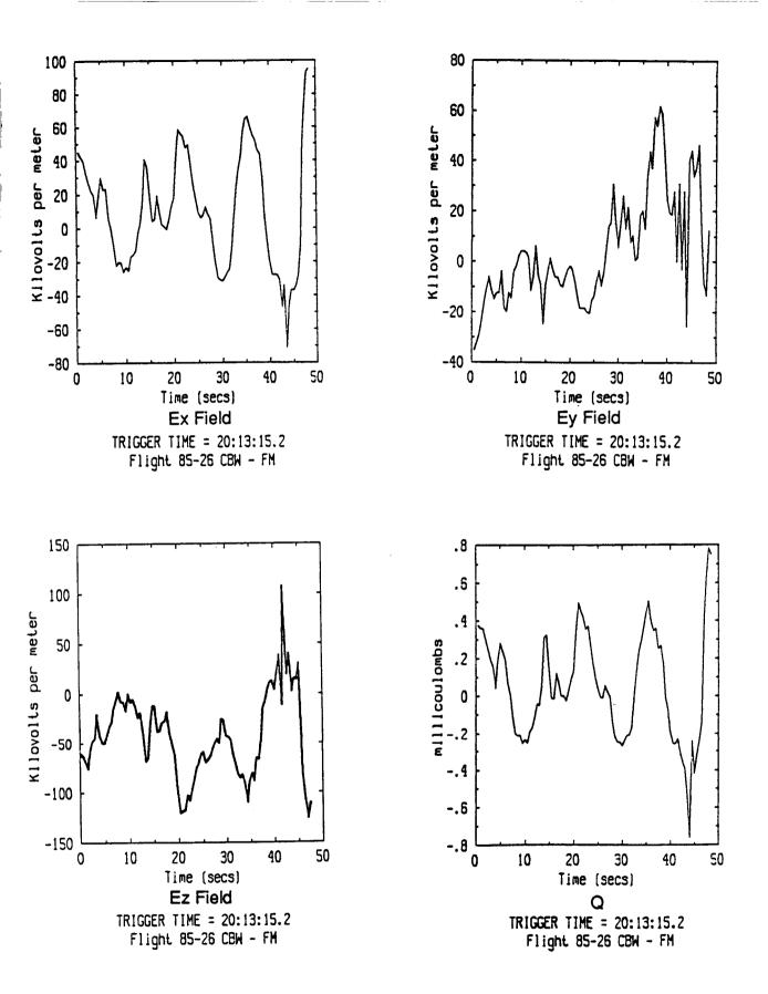
Figure 3.3a Calculated Ambient Fields Just Prior to the Strike for the Coarsely Modeled F106B (Strike Time Is at 48 Seconds)
