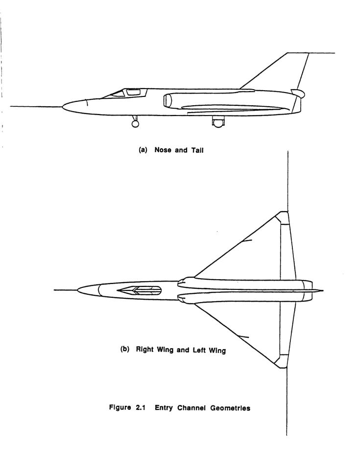
The numerical results indicate that from the 27 strikes analyzed, 20 fall into the category of nose attachments, 3 were left wing attachments, 3 were right wing attachments and a single tail attachment case is probable for Flight 85.035 Run 005 Strike 005. The large percentage of nose attachments witnessed in the measured data once again confirms the high probability of channel formation at this particular location on the F106B.
