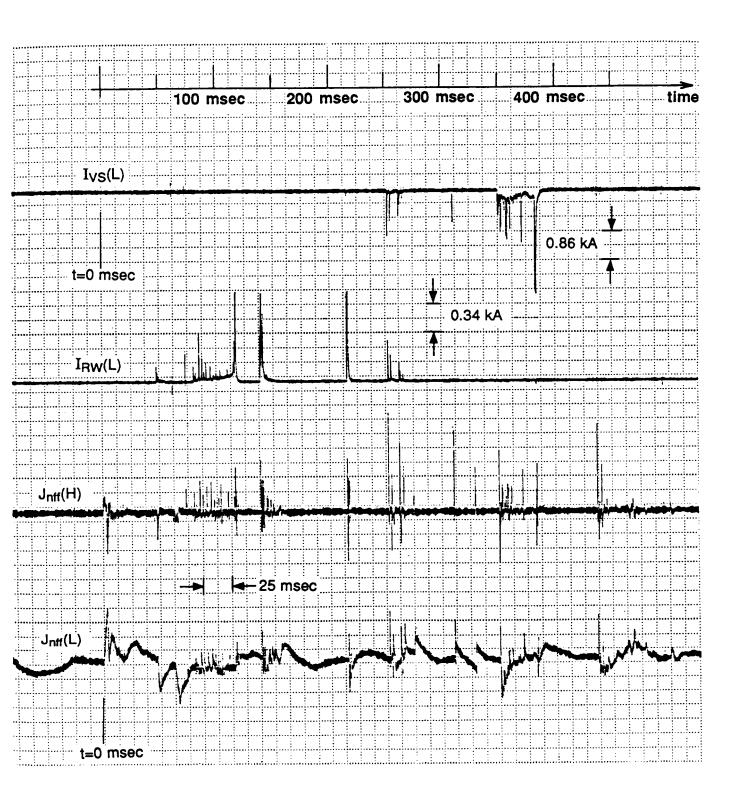
Figure 5.5 E-Field and Current Sensor Records from Flash 4, 4 August 1987
