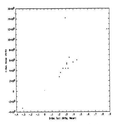
Figure 2.7 Peak Value Scatter Diagram 5 Derived from 1985 Measured I-dot and D-dot Tail Response Data
