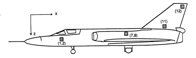
Figure 4.3 Side View of F106B Showing Test Point Locations
