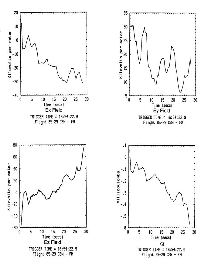
Figure 3.7a Calculated Ambient Fields Just Prior to the Strike for the Coarsely Modeled F106B (Strike Time Is at 28 Seconds)
