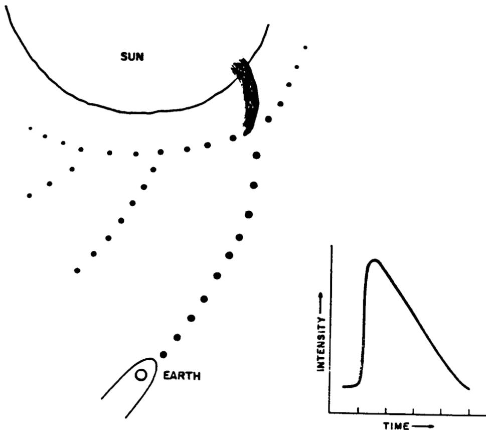
Figure 5. Graphic representation of particle propagation along the interplanetary magnetic field line from the sun to the earth from a solar flare at the "footpoint" of the field line. The larger the dot, the larger the flux. A typical intensity/time profile for this event, as measured at the earth, is shown on the right.
