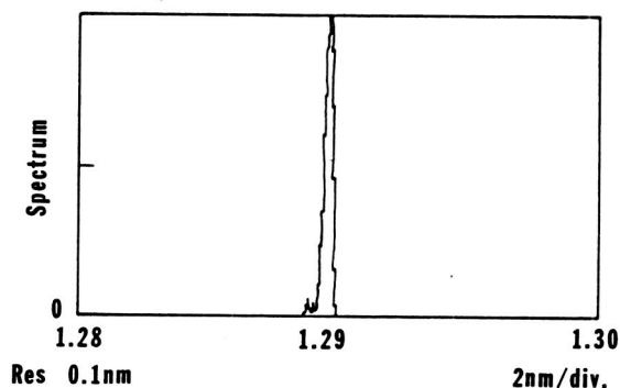
Figure 18. Spectral output from a gain-guided DBR-LOC laser.
