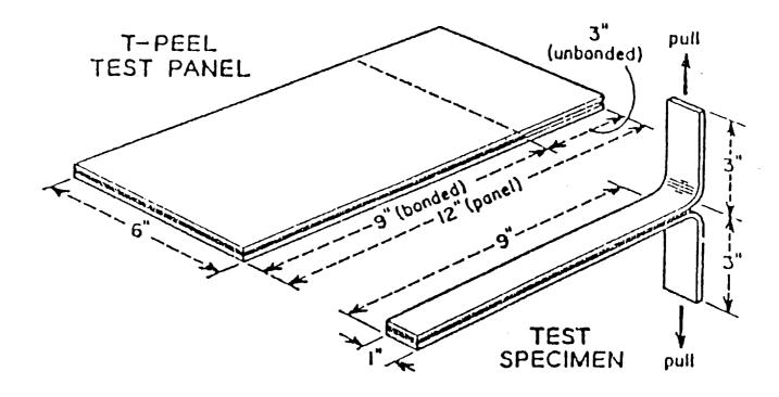
Figure 3. Peel Strength Specimen
