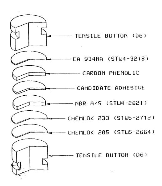
Figure 4. Tensile Button Configuration
