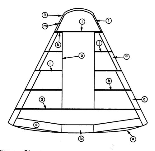
Figure 34. Capsule Structural Parts Identification.
