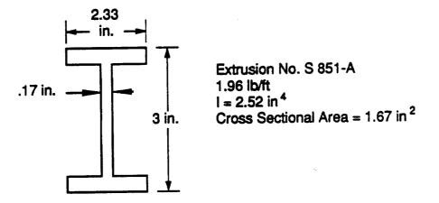
Figure 36. Extrusion No. S 851-A Dimensions and Properties.
