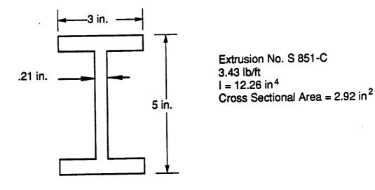
Figure 35. Extrusion No. S 851-C Dimensions and Properties.
