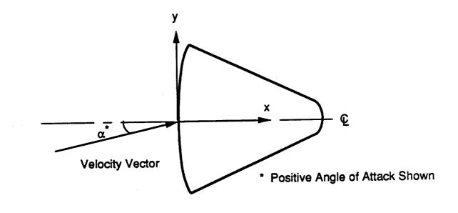
Figure 9. Reentry Capsule Angle of Attack and Coordinate System.
