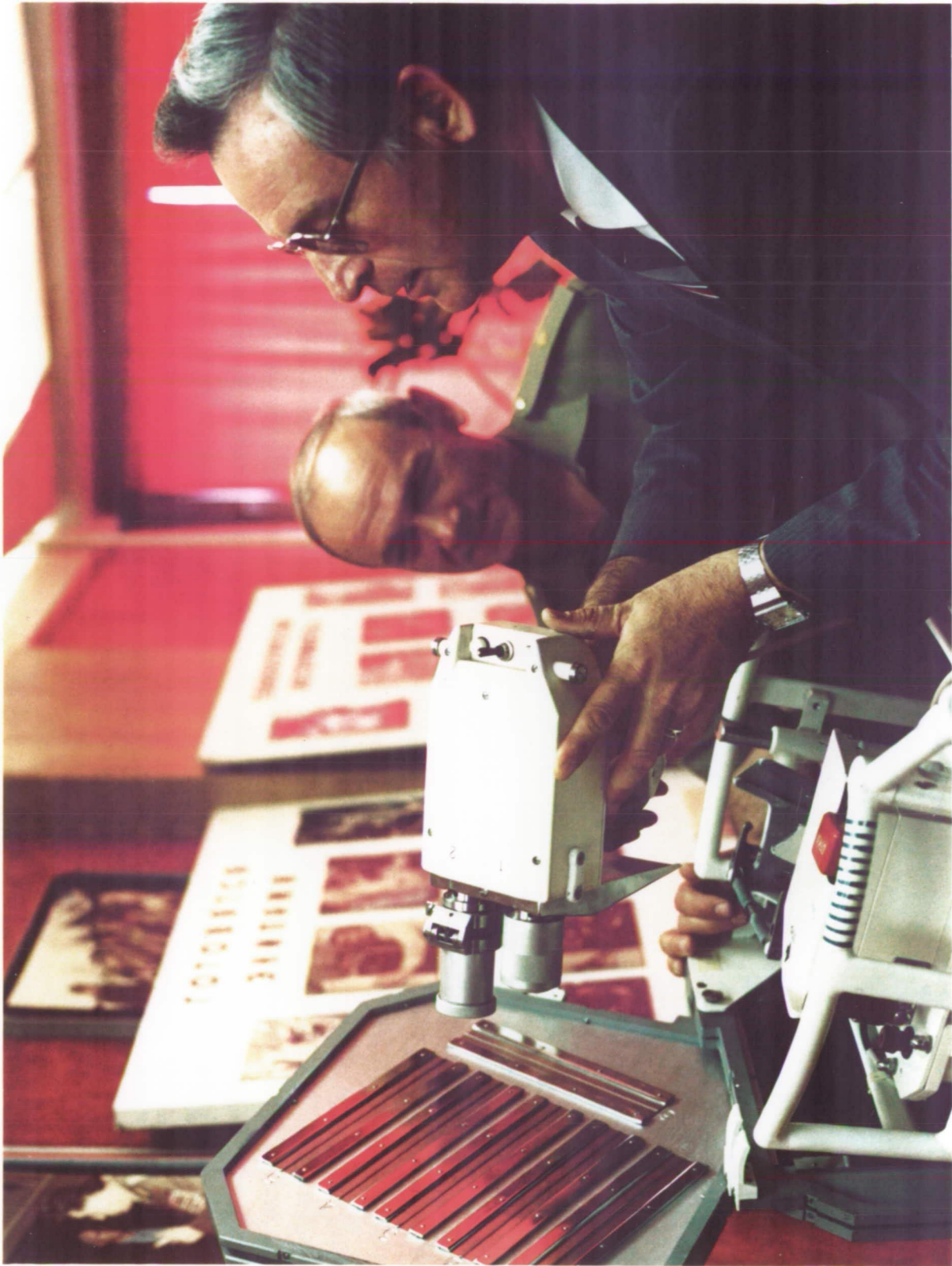
Figure 40. Rocketdyne representative Hal Conaway discusses Soviet multi-purpose electron-beam device with cosmonaut Major General Vladimir Djanibekov. Major General Djanibekov worked with this device during the EVA Welding Experiment performed in July 1984.
