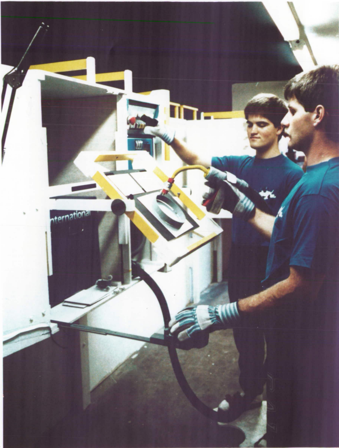
Figure 31. "Test Subject Crewmember" Welding in the 45-Degree Chest-Level Orientation During the Time Line Simulation of Task 5
