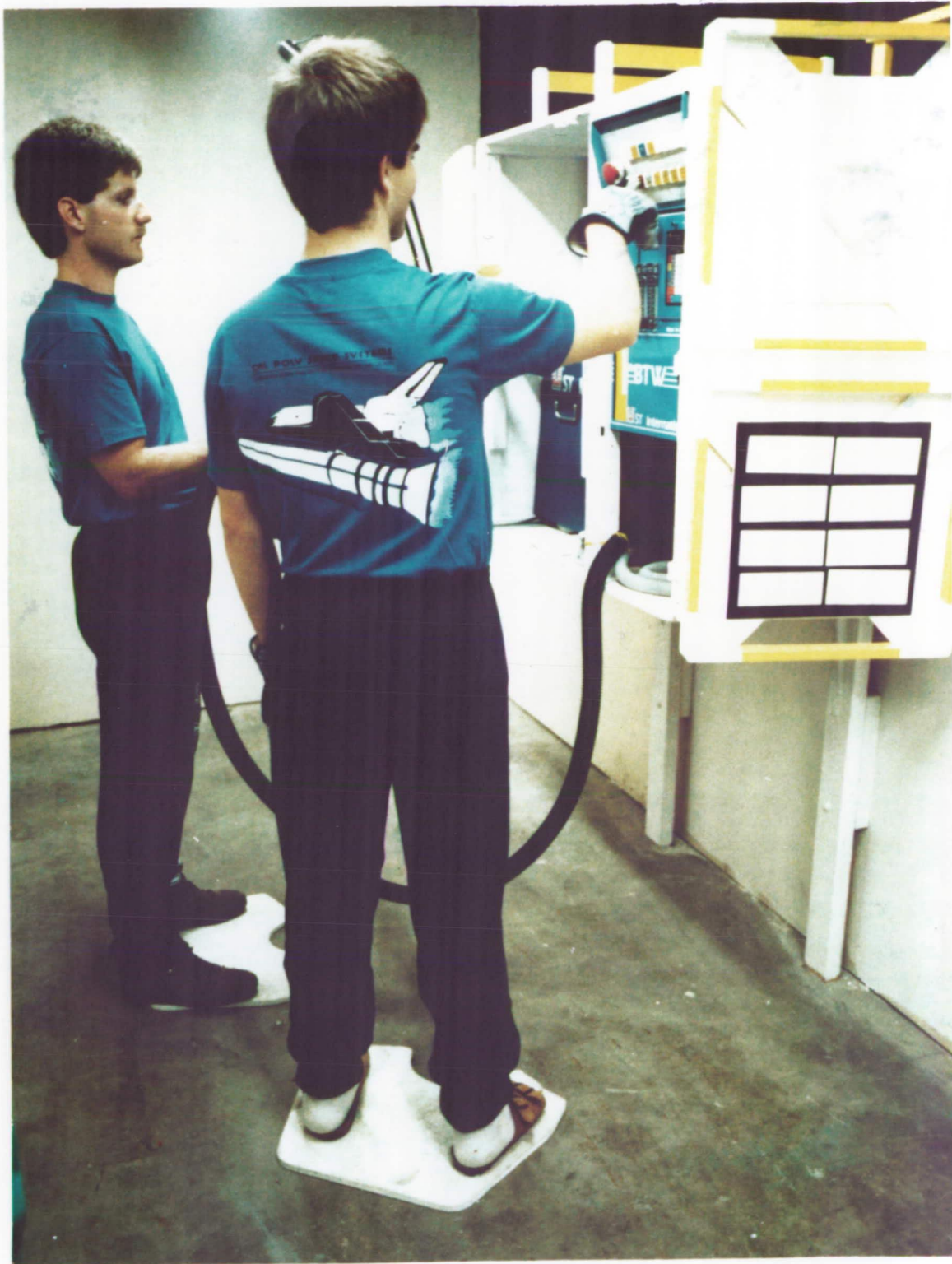
Figure 29. Relative Orientations of the "Test Subject Crewmember" (Left) and the "Supporting Crewmember" (Right) in Foot Restraints at the Welding Station During Time Line Simulation
