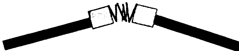
Figure 4.3 One Piece Flexible Coupling
